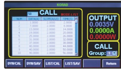
The spreadsheet embedded in the LCD , easy to do the output sequences and data settings
